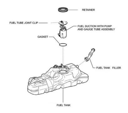
32.4 The fuel pump module hosts the fuel pump, associated plumbing and the fuel gauge sending unit. The fuel pump module drops into the fuel tank through an access hole on the topside of the tank. A retainer ring ensures that the flange and O-ring create a tight seal against the tank surface, preventing fuel escape:
