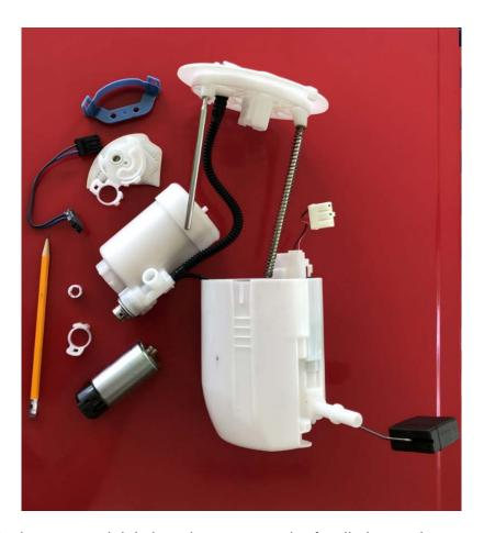
32.5 The fuel pump module's housing protects the fragile internal components that fit together very specifically within the module and is held together with plastic tabs and clips:
