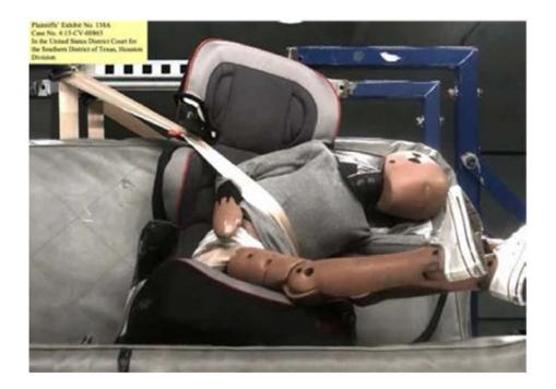
56. The same technician has stated that, in 13 years, he did not once perform a "failed" side-impact test on a booster seat. He also testified that the following images—all of which are from "passed" Evenflo side-impact tests, and use a dummy based on a three-year-old child would have been ticked as "yes":
